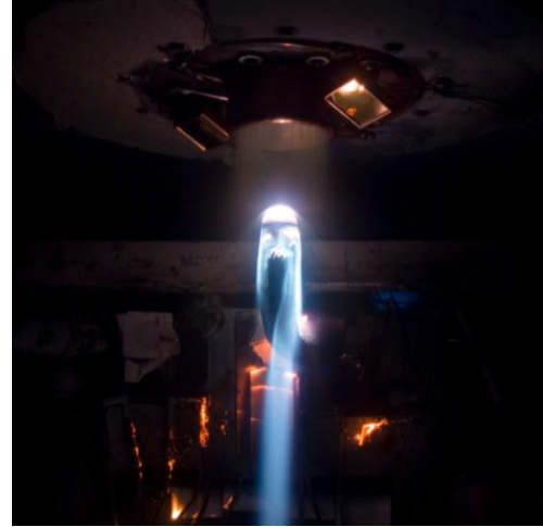
Figure 8. Top view of the IHF test cabin during a TPS test run.
