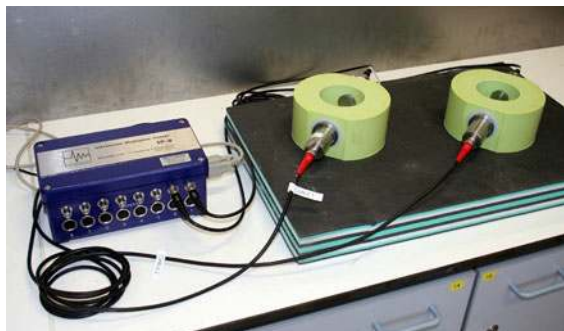
Fig. 3 The complete multi-channel IP-8 continuous ultrasonic testing device in a 2-channel setup
