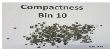
(b) Kimberlitic material sorted based on compactness in the range of 0.81 to 0.85; -8+2.8 mm material
