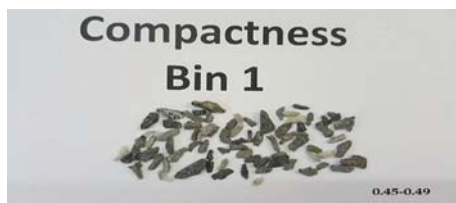
(a) Kimberlitic material sorted based on compactness in the range of 0.45 to 0.49; -8+2.8 mm material
