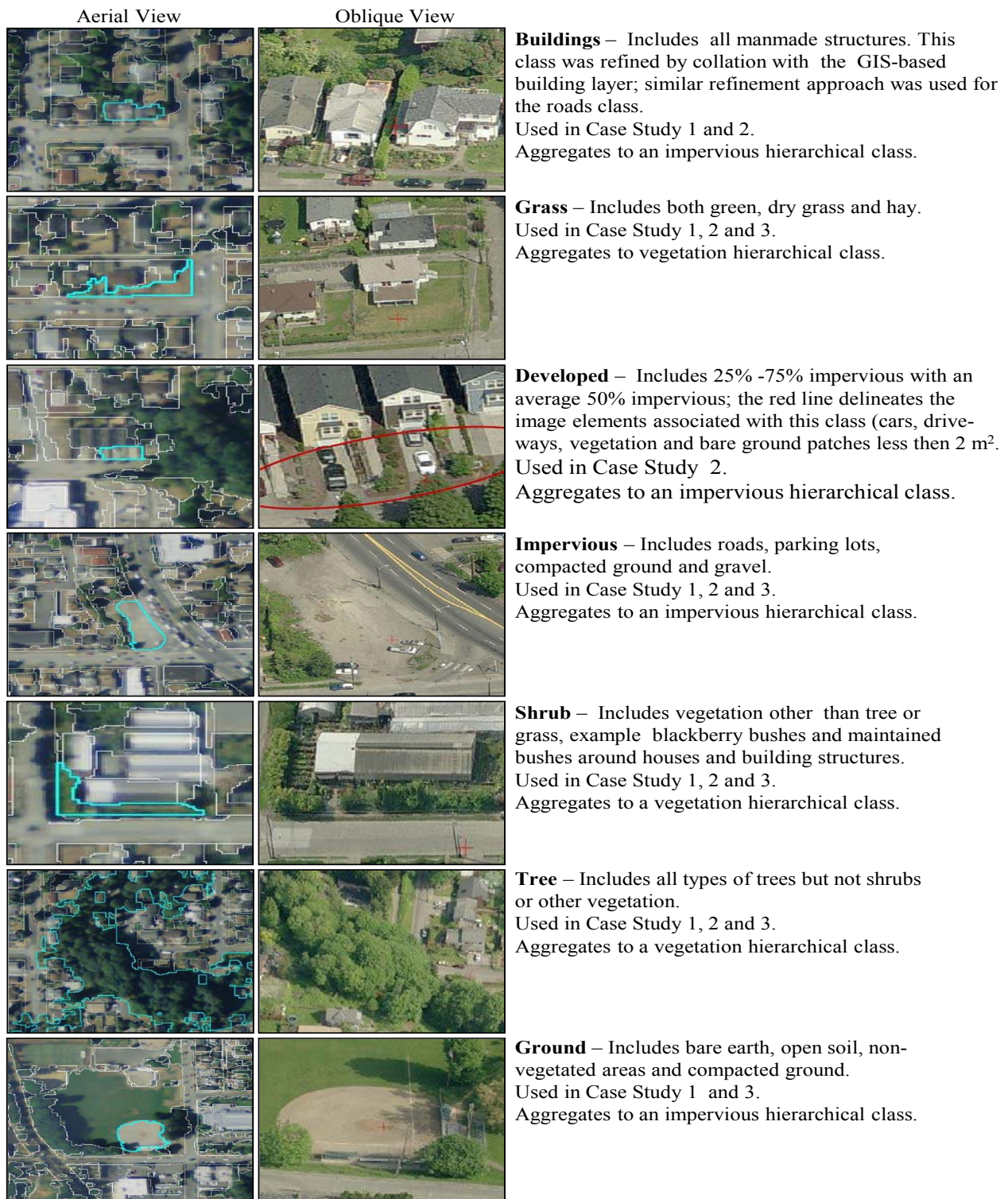
Figure 2. Example of image segments representative of the described LULC classes. Cyan polygons show an example of the LULC class being delineated in the OBIA segmentation, adjacent segments are shown in white and can represent a different class. The oblique image is centered on the delineated segment. The 2002 aerial and co-registered 2009 oblique images are not shown at the same scale; north is up.
