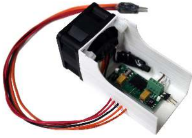
Figure 15: Temperature sensitivity test setup. An instrumented version of Monjolo's power supply is housed in a temperature-controlled enclosure. A fan at the rear ensures constant airflow and an analog temperature sensor between the power supply and the fan measures the temperature near C_{store} .
