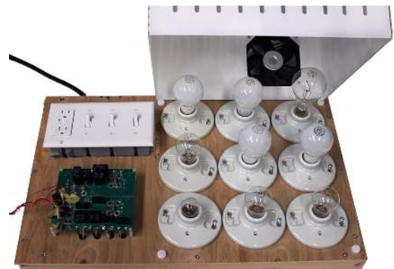
Figure 7: Calibration testbed. A control board manages nine circuits of light bulbs and power resistors with varying wattages. The values are chosen to allow for 1 W steps in load power. Light switches provide a hard shutoff, but during experimentation, wattages are selected via relays controlled by an Epic Core on the control board shown in the bottom left. The load is independently metered by a PLM-1LP for ground truth.
