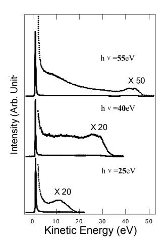
**Figure S3.** Photoelectron spectra of [121]6-tetramantanethiol SAMs on Ag collected with 25 eV, 40 eV, and 55 eV photon energy. The unusual electron emission peak at 1 eV persists. A quantitative analysis of the peak intensity upon photon energy is non-trival because of the unavoidable higher harmonic components of synchrotron photon beam.
