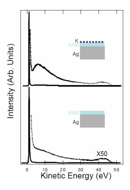
**Figure S4.** Photoelectron spectra of [121]6-tetramantanethiol SAMs with (upper) and without (lower) potassium deposition. No energy shift was observed for the sharp peak, and only a small increase of the secondary electron background can be seen.
