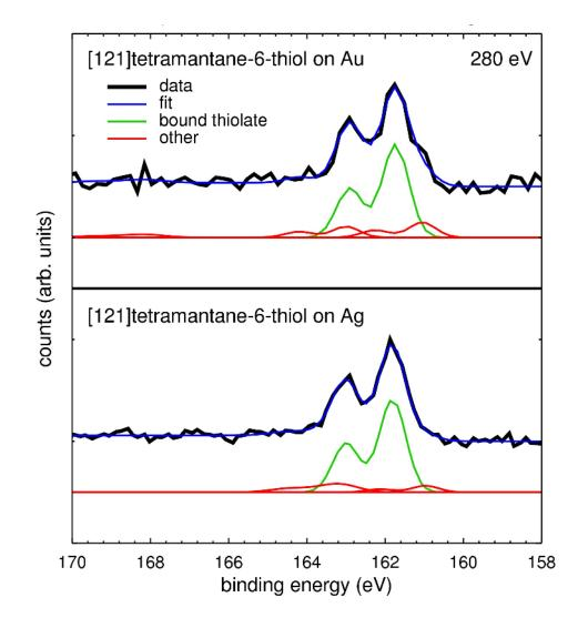
Figure S2. Black lines are S 2p core-level X-ray photoelectron spectra (XPS) of [121]6-tetramantanethiol SAMs on Au (top panel) and Ag (bottom panel). Blue lines are fittings to the data based on Au-thiolate and Ag-thiolate sulfur (gree lines). Other S species, unbound, elemental, and oxidized sulfur, only have insignificant contributions (red lines).
