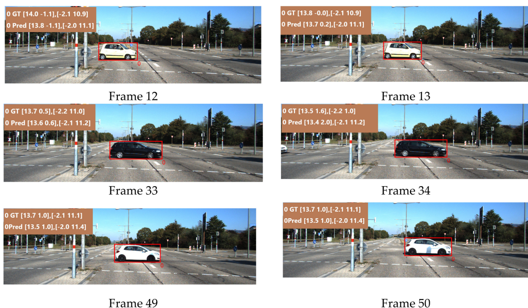
Figure 8. Prediction results of the target vehicle in the lateral incoming vehicle scenario.
