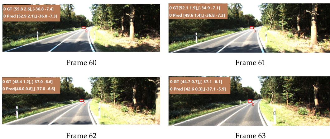
Figure 10. Prediction results of the target vehicle in the opposite direction traffic scenario. The green font represents the true values, which are the longitudinal lateral distance and longitudinal lateral velocity; the blue represents the predicted values, which are the longitudinal lateral distance and longitudinal lateral velocity.
