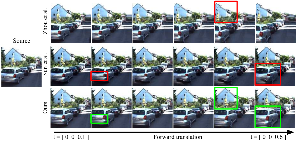
Figure 5: Simple camera motion. Setting: Given a source view we synthesize linear forward motion over 0.6m. Our method produce sharp and correct images while [62, 51] produces distorted images. Zhou et al. [62]’s motion is incorrect, while Sun et al. [51] stays stationary. Ours reflects a reasonable straight forward transition.
