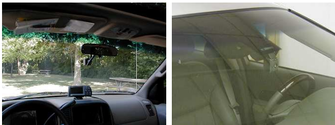
Fig. 1. Low light camera in the prototype vehicle
