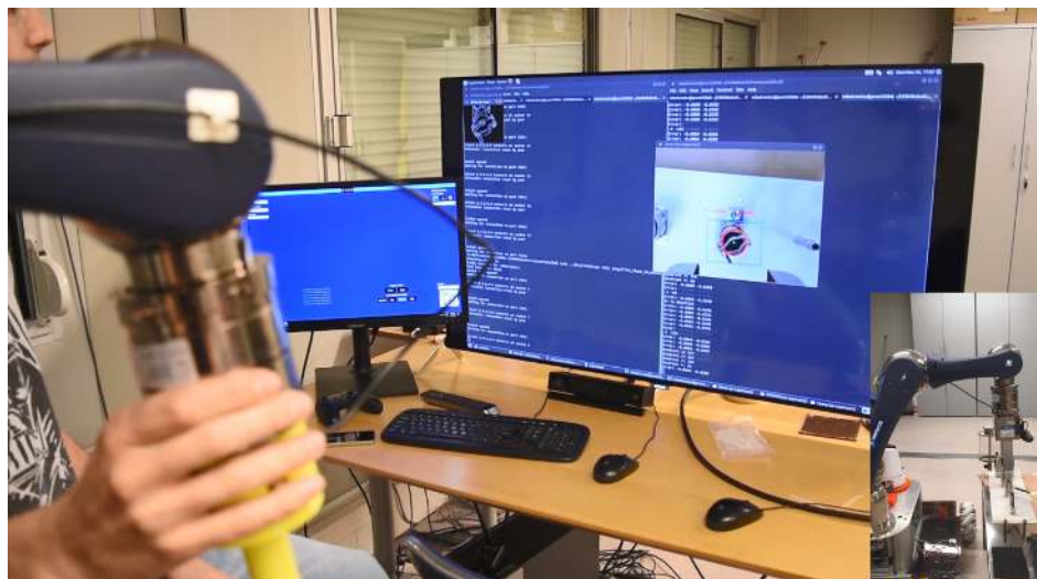
Figure 13. Operator guidance by tracking-based Depth Estimation system upon metallic surface.
