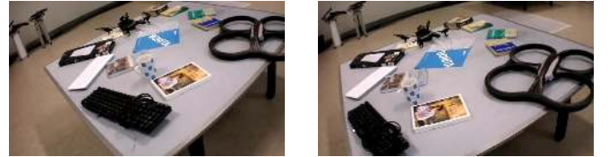
Fig. 7. The video is discontinuous at frame 508 and 509 due to the frame loss caused by unstable Wi-Fi link
