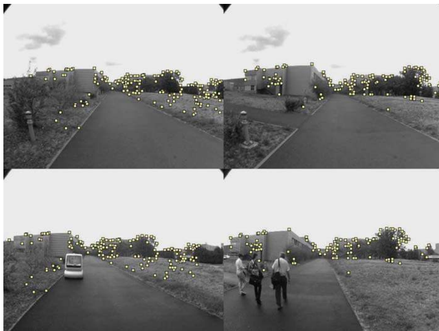
Figure 24. Interest points correctly matched between the reference key frame and the current image. Left: when the robot is nearly on the learning path. Right: when the lateral deviation is maximal. The reference frame is on top.
