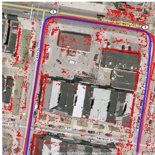
Fig. 6. 3D points overlay on the satellite image for the 2.5 km sequence (figure 5b)
