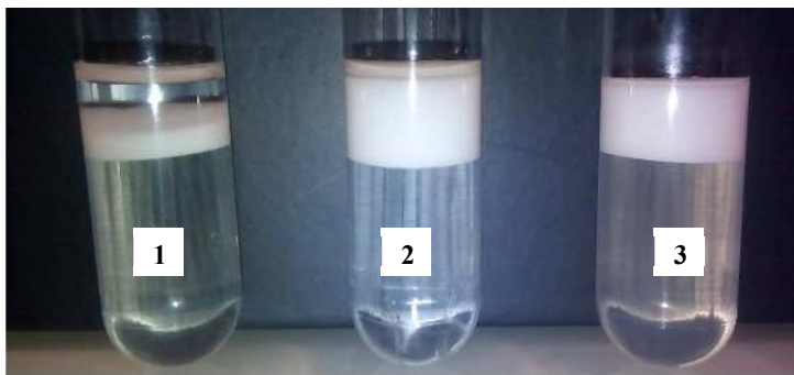
Figure 9. Stability under centrifugation for an emulsion initially prepared with 0.5 wt.% NaCAS. (1) Not supplemented; (2) supplemented with 2 wt.% NaCAS and rinsed; (3) supplemented with 2 wt.% NaCAS, unrinsed.
