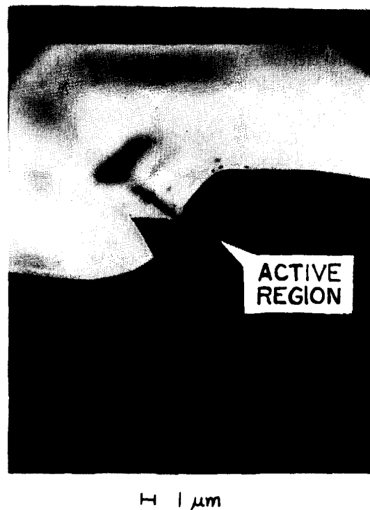
FIG. 2. SEM picture of the groove laser.
