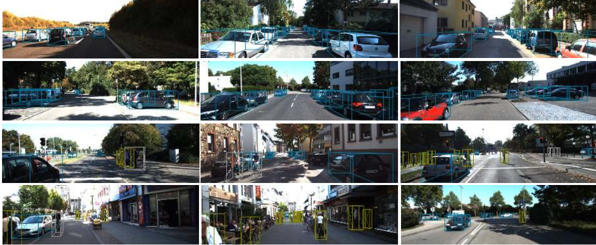
Figure 7: Qualitative results in KITTI validation set. Cyan, yellow and grey mean predictions of car, pedestrian and cyclist.
