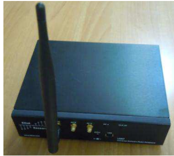
Figure 11. The software-defined radio (SDR) platform used in the experimental tests of the RF-to-DC conversion efficiency.
