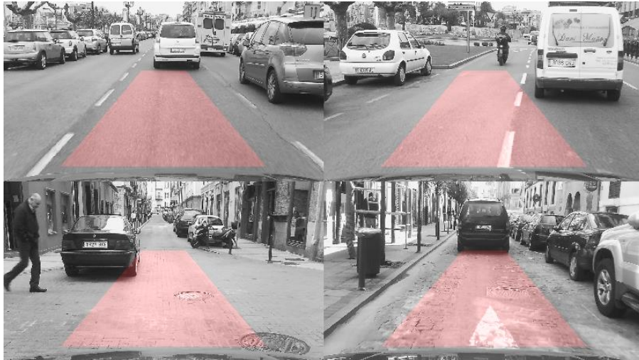
Fig. 1. Vehicle's search area (ROI) corresponding to the safety area.
