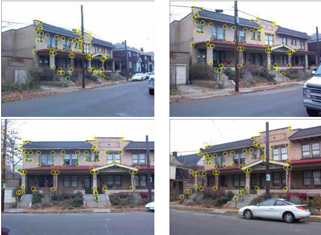
Figure 1.2: Structure from motion example. The goal is to estimate the 3D structure and the camera location associated with the images (4 out of 5 images shown).
