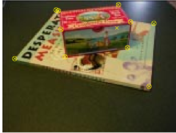
Figure 8.3: Image 1 of the “book” sequence with the measurements and the MAP estimate superimposed. Note that the position of the occluded corner of the box is predicted but a measurement is not available due to occlusion.
