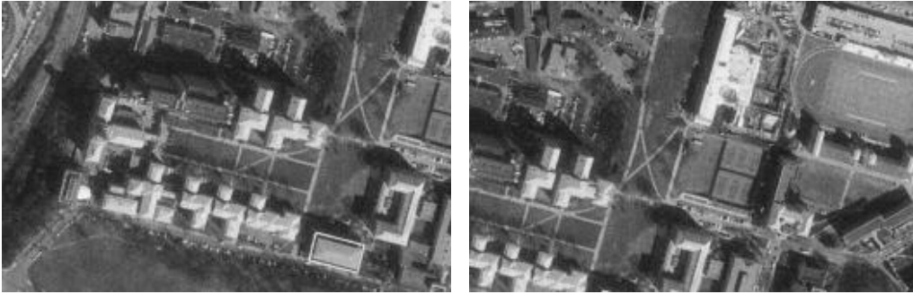
Figure 1.1: An instance of a 2D image registration problem: the goal is to estimate the translation between the two images (images courtesy of the US Geological Survey).
