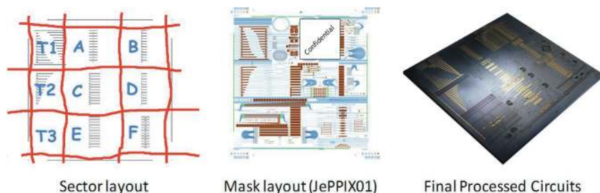
Figure 4 (online color at: www.lpr-journal.org ) Example of a Multi-Project Wafer (MPW) realised in the JePPIX01 process. The wafer is subdivided in 9 sectors, three for test structures and 6 for user designs. The picture in the middle is an example of a mask layout, and at the right is a photograph of the realised wafer.
