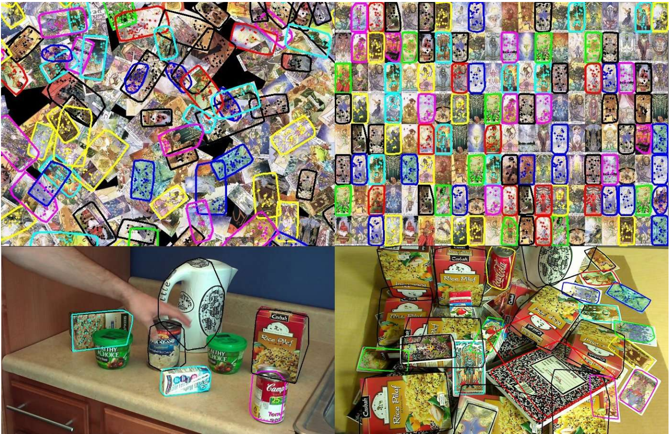
Fig. 4. MOPED Benchmarks. For the sake of clarity, only half of the detected objects are marked. (a) The Rotation Benchmark: MOPED processes this scene 36.4x faster than POSESEQ. (b) The Zoom Benchmark: MOPED processes this scene 23.4x faster than POSESEQ. (c) The Simple Movie Benchmark. (d) The Complex Movie Benchmark.
