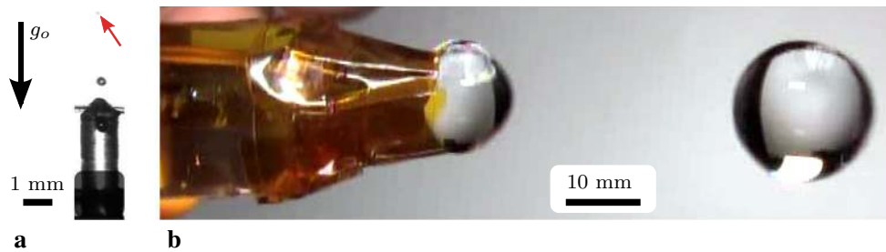
Fig. 3 Sample breadth of auto-ejection from tests performed at (a) 1 g and (b) aboard the International Space Station (ISS). a A 1.7 nl PDMS droplet (arrow) ejected at 1.12 m/s followed by a 36 nl droplet ejected at 0.106 m/s on bench top terrestrial experiment using small
