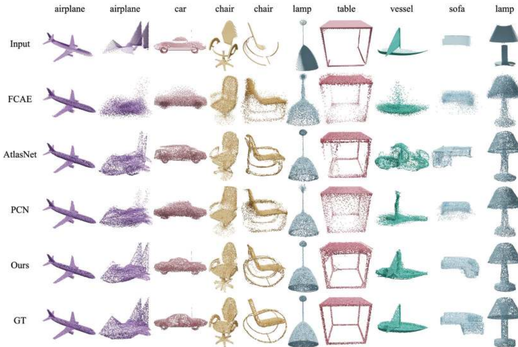
Figure 7: The figure shows the completion results of different methods. Each output point cloud consists of 8,192 points.
