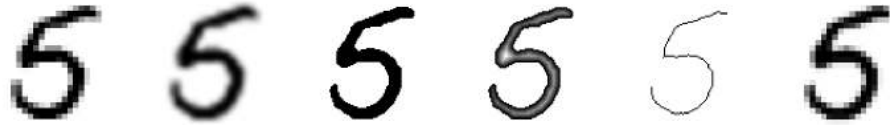
Figure 2: Stages of the image processing pipeline. Left to right : original image, upscaled image, binarised image, distance transform, skeleton, downscaled image.
