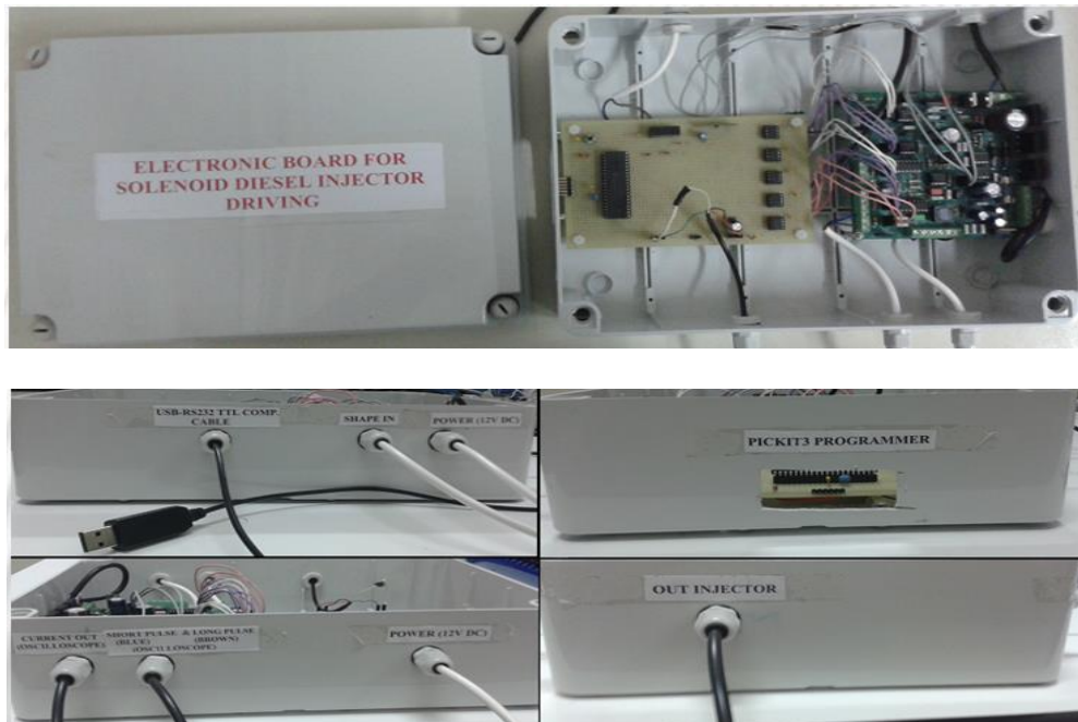
Figure 12. Final aspect of the injectors driving unit placed into a branch box: rubberised bipolar cables were used for connecting the realised electronic system with the outside.
