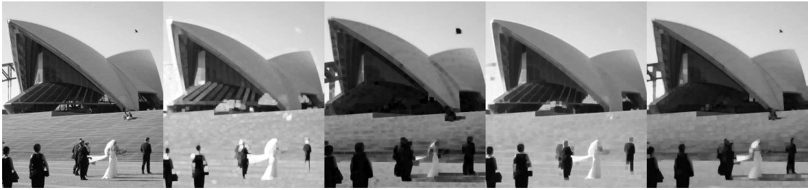
Figure 1: Original image (opera), dilation, erosion, closing and opening with a 21 \times 21 square.
