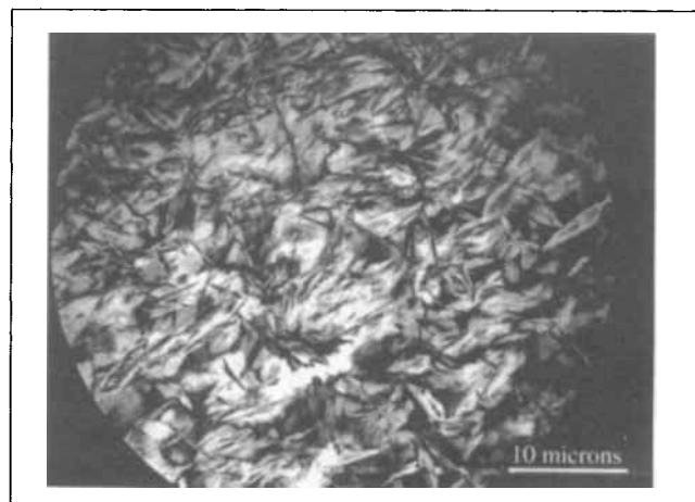
Figure 2. Microscopic image of the incipient gel layer deposit in a flow cell under a laminar flow.
