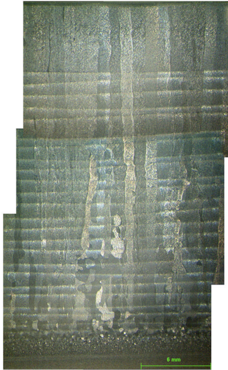
Fig. 6 Montage of macrostructure of GTAW deposition Ti6Al4V wall with direct current 195A, travel speed 0.54m/min, and wire feed speed 3.2m/min shows large columnar growth prior beta grains, the scale bar is 6mm
