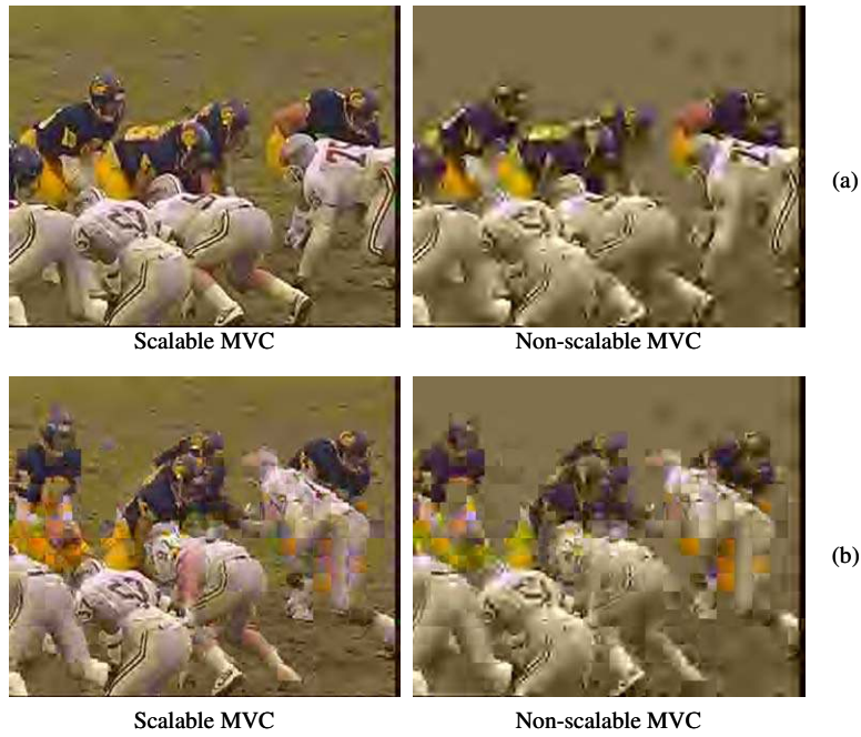
Figure 8: Comparison between scalable and non-scalable MVC employed in the codec of [6]: Visual comparison for the “Football”-sequence decoded at 192 kbps. (a) Frame 0. (b) Frame 8.
