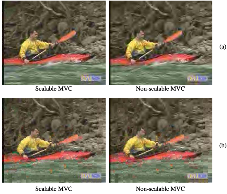
Figure 9: Comparison between scalable and non-scalable MVC employed in the codec of [6]: Visual comparison for the “Canoa”-sequence decoded at 256 kbps. (a) Frame 0. (b) Frame 2.
