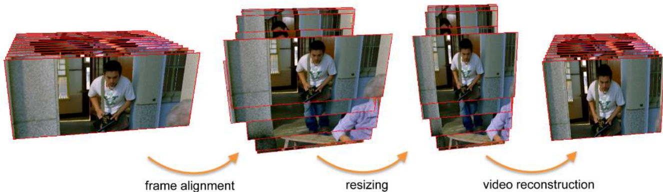
Figure 1: Overview of our automatic content-aware video resizing framework. We align the original frames of a video clip to a common coordinate system by estimating interframe camera motion, so that corresponding components have roughly the same spatial coordinates. We achieve spatially and temporally coherent resizing of the aligned frames by preserving the relative positions of corresponding components within a grid-based optimization framework. The final resized video is reconstructed by transforming every video frame back to the original coordinate system.
