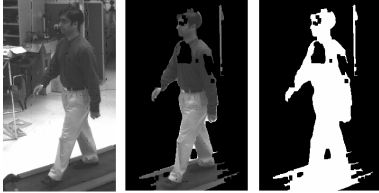
Figure 2. From left-to-right: original image, foreground template and binary template, of a walking person.
