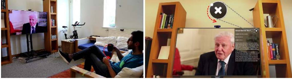
Fig. 12. Tracematch is designed for casual motion input. A camera tracks any motion in the front of the screen and correlates it with on-screen moving control. This enables users to provide input with any part of their body, and regardless of their posture. In this scene, the user is able to close a pop-up screen on the TV by mimicking the widget’s motion with his hand even though he is holding a drink.
