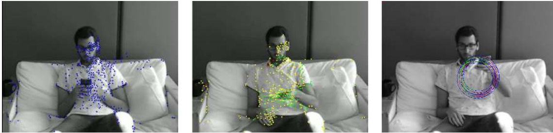
Fig. 13. TraceMatch processing pipeline. (A) Features detected from FAST and previous optical flow iteration. (B) Candidate features (green) and non-candidate features (red). (C) Features below the Pearson product-moment correlation coefficient threshold (red), features above the threshold (green), and the first feature to be matched is shown with its trajectory and the fitted circle from RANSAC (blue).
