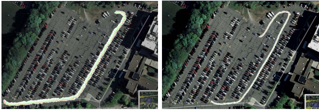
Fig. 9. Estimated camera motions using the spherical model.
