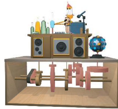
Figure 10: Editing on the Robot DJ toy. Part's drawn in brown were updated according to the user's edit. Please see the accompanying video for the entire editing session.
