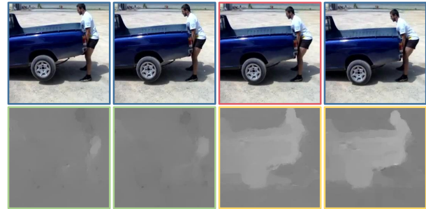
Figure 1: Best viewed in color. Example video frames shown with optical flow in the bottom row. The frame in red box is the sampled key frame. The flow images in green and yellow boxes are the horizontal and vertical component of the optical flow computed around the key frame, respectively.
