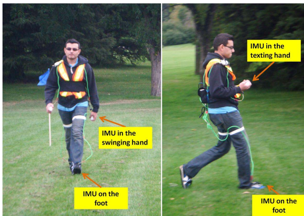
Figure 11. (Left) Test subject walking with the IMUs in his swinging hands; (Right) Test subject walking with the IMUs in his texting hands.
