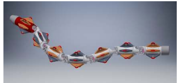
FIGURE 16. Complete model of the multi-joint snake-like robot.
