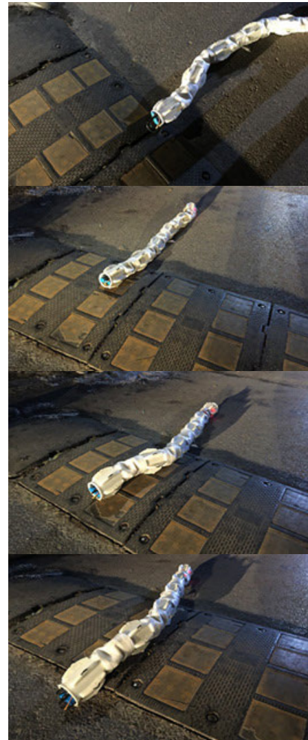
FIGURE 33. The multi-joint snake-like robot crossing the deceleration belt.
