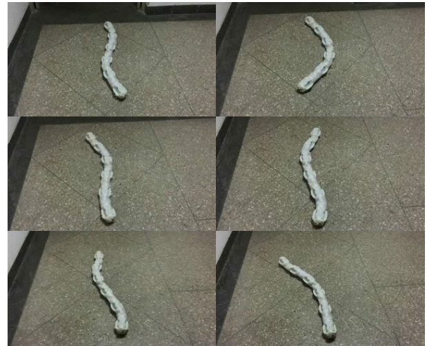
FIGURE 27. The multi-joint snake-like robot moving on the floor of corridor.
