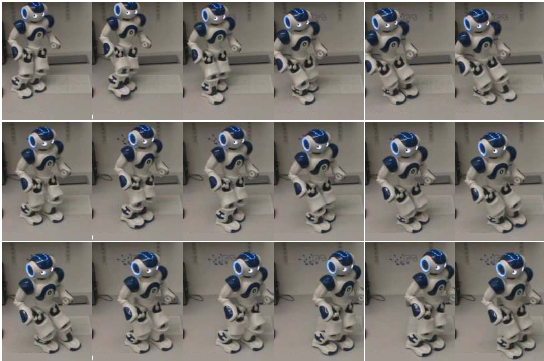
Figure 4.12: An example of a generated walk from random feet start and end-point positions. The generated walk is stable and relatively fast while the possible reach of the steps is greater than the standard motion synthesis procedure from Aldebaran Robotics. Additionally the motion generation is fast and can be employed in an online motion planner.
