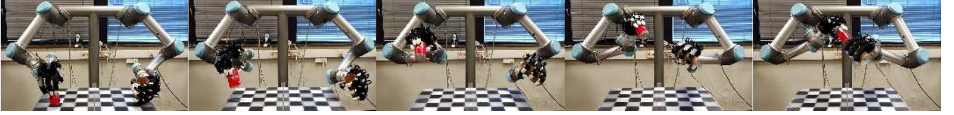
Fig. 6. Snapshots of a solution path for the assembly example planned in the reduced subspace B_k .
