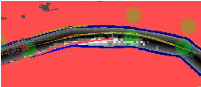
Fig. 6. Planning along a lane that becomes increasingly narrow due to detected curbs (red line emerging into the lane on the bottom). The motion planner is still able to find feasible trajectories that follow the road curvature.
