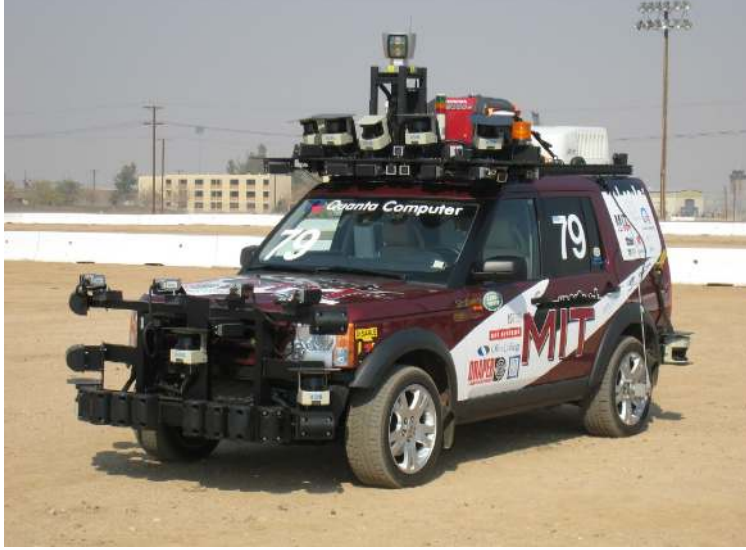
Figure 12. Talos: Team MIT's race vehicle at the DARPA Urban Challenge
