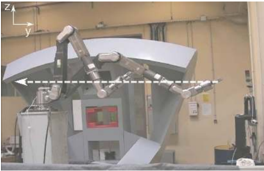
Fig. 9 Views of the robot in initial position (extended) and at t = 5.0s (fold up). The white arrow is the constant operational desired velocity from t = 0.0 s to t = 5.0 s
