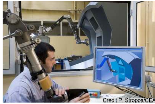
Fig. 8 Teleoperated Maestro operating in front of the tunnel boring machine cutting wheel mockup
