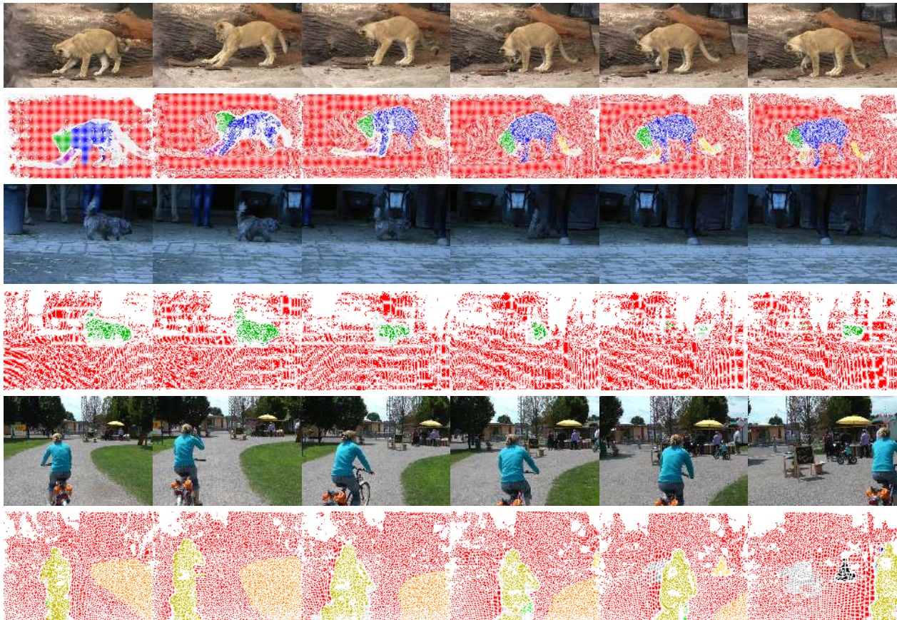
Figure 5. Frames 1, 20, 40, . . . , 100 of the lion01 sequence, frames 80, 100, . . . , 180 of the dogs01 sequence and frames 120, 140, . . . , 220 of the people05 sequence of FBMS-59 and the results of our MCE motion trajectory segmentation. Articulated motion can lead to a slight overegmentation as in the lion01 example (top). In the dogs01 sequence (center), the dog is correctly tracked despite the occlusion. The people05 sequence (bottom row) shows the effect of a moving camera. While the moving objects in the scene (adult biker, child on the balance bike) are segmented, some static objects are segmented as well, as for example the blackboard.
