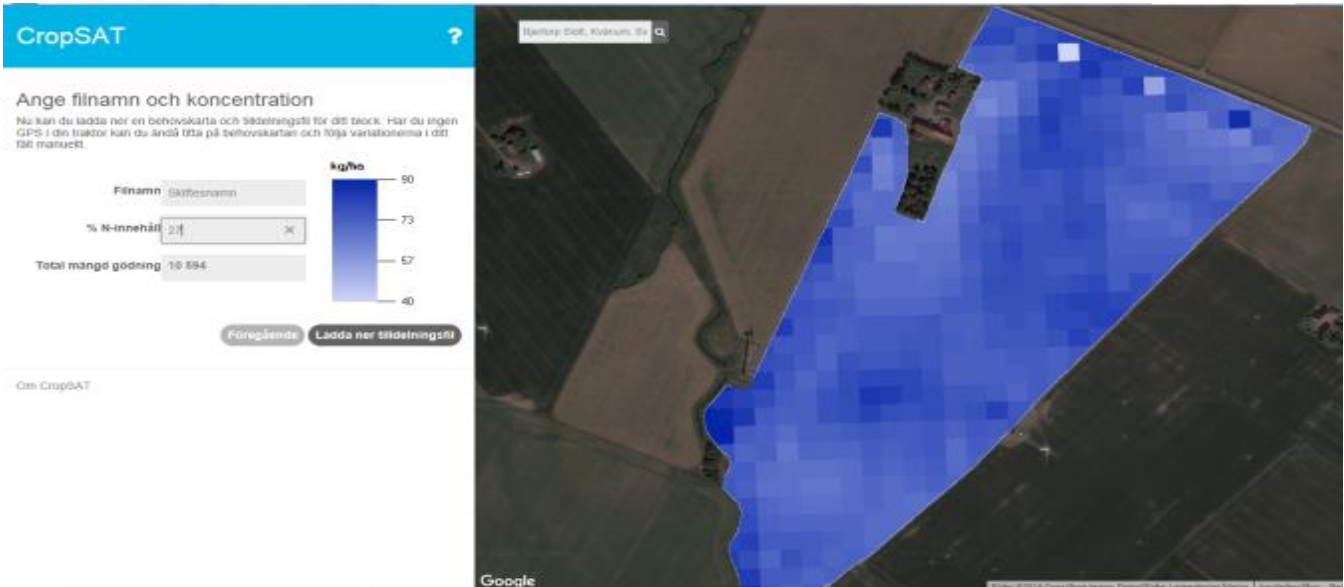
Figure 1b. A variable rate application (VRA) file ready to be entered into the fertiliser spreader via a USB memory stick.
