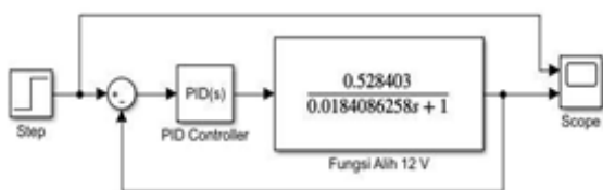
Fig. 5. Simulink block diagram of the PID system
