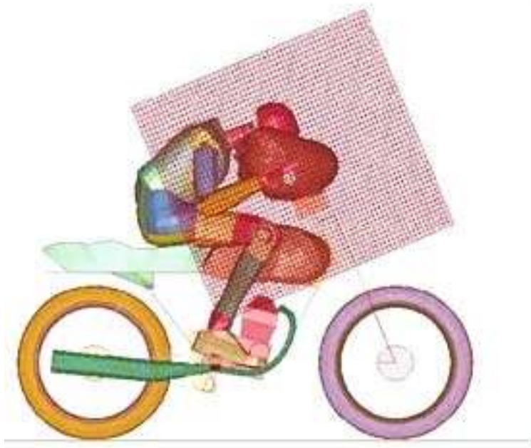
Figure 12. A typical inflated state of the motor cycle and the airbag.
