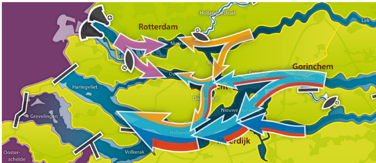
Figure 11a: schematic representation of the river water flows during a storm surge. The added effect of climate change and/or higher flood standards spreads out over different branches.
