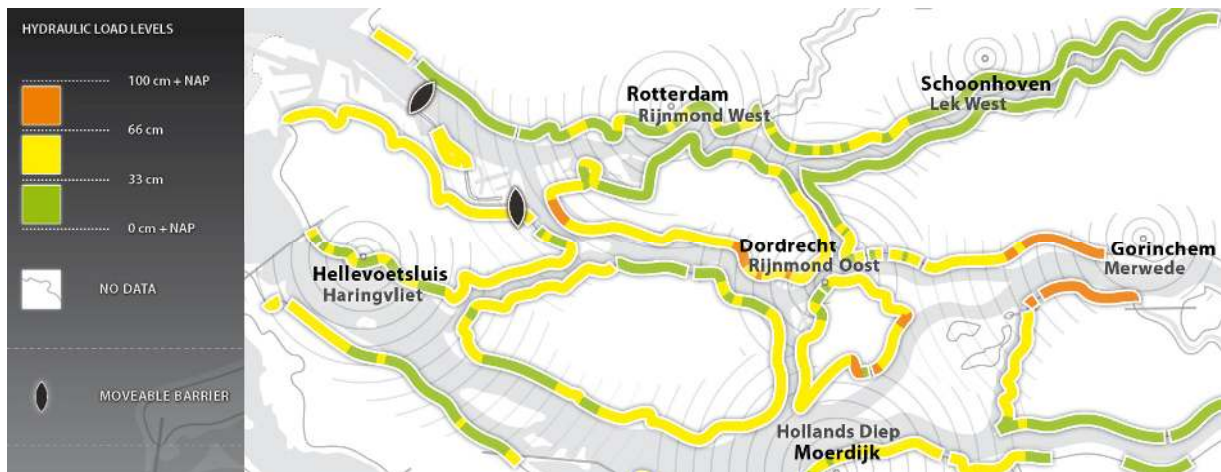
Figure 6: Increase of 'hydraulic load levels' (design water levels also incorporating the wave run) under the 'G+' - climate scenario in 2100 (65 cm sea level rise and 12,5% more river discharge), without additional moveable river barriers, at a failure rate of the Europoort barrier of 1/100, under the current safety standards.
