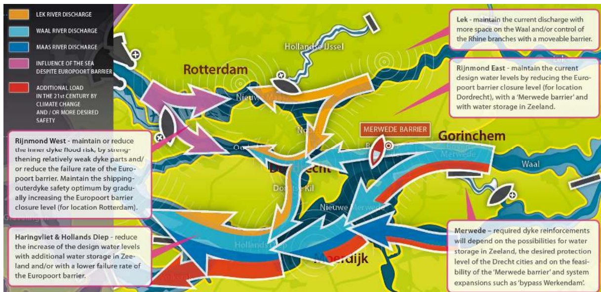
Figure 11b: vision for short term measures based on this research. The added effect of climate change and/or higher flood standards is directed towards the eastern and southern rural area, limiting the effects on the urbanised northern area.
