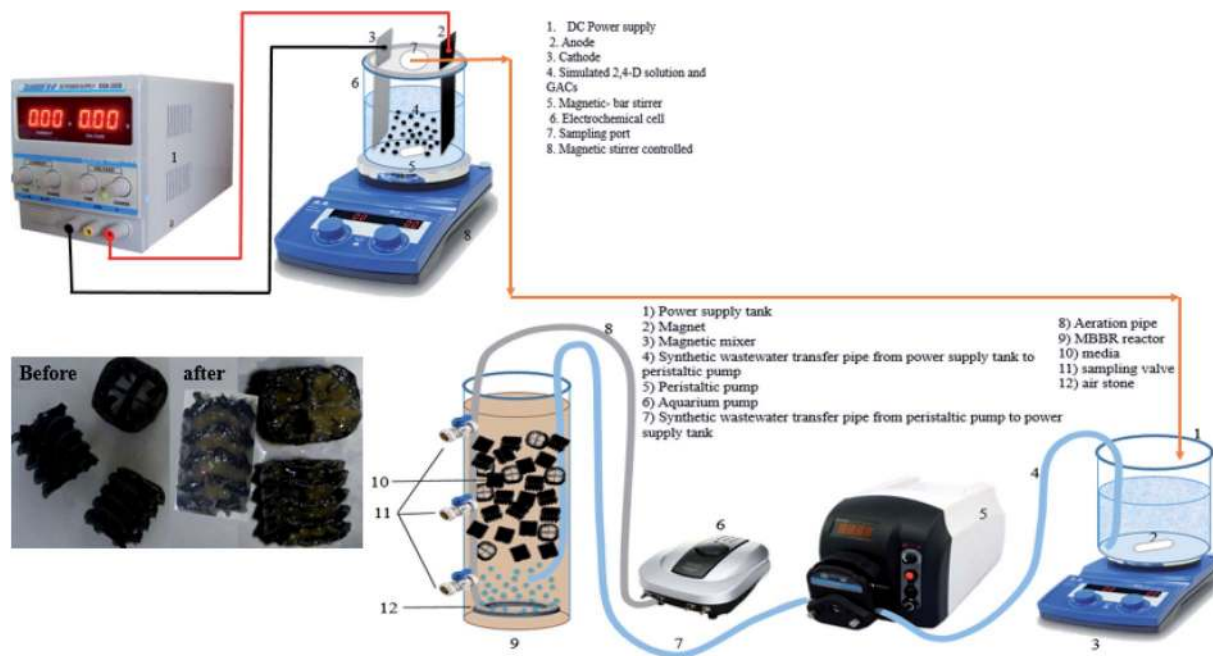
Fig. 1 Schematic of reactor used in this study.
