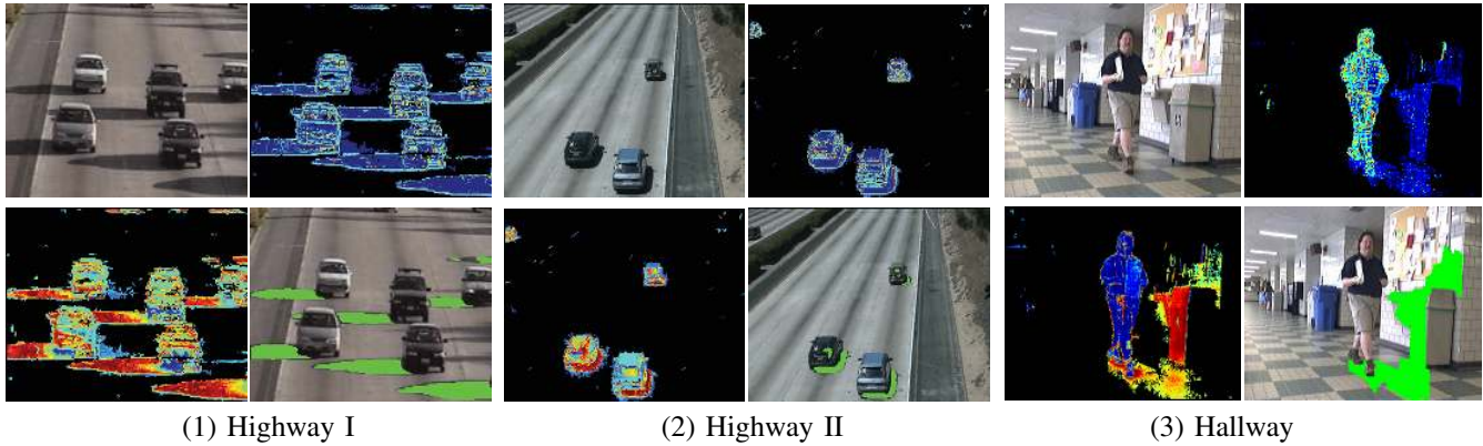
Figure 5. Visual results in various environments. \frac{a|b}{c|d} (a) Frame from video sequence. (b) Hamming distance of SILTP. (c) Likelihood probability in color space. (d) Final result using MRF
