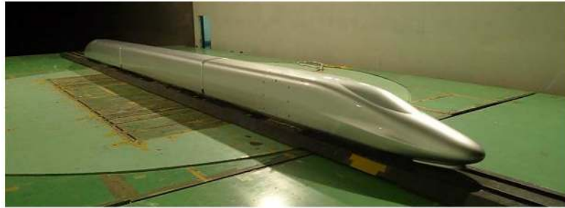
Fig 10. Train model in the tunnel.
